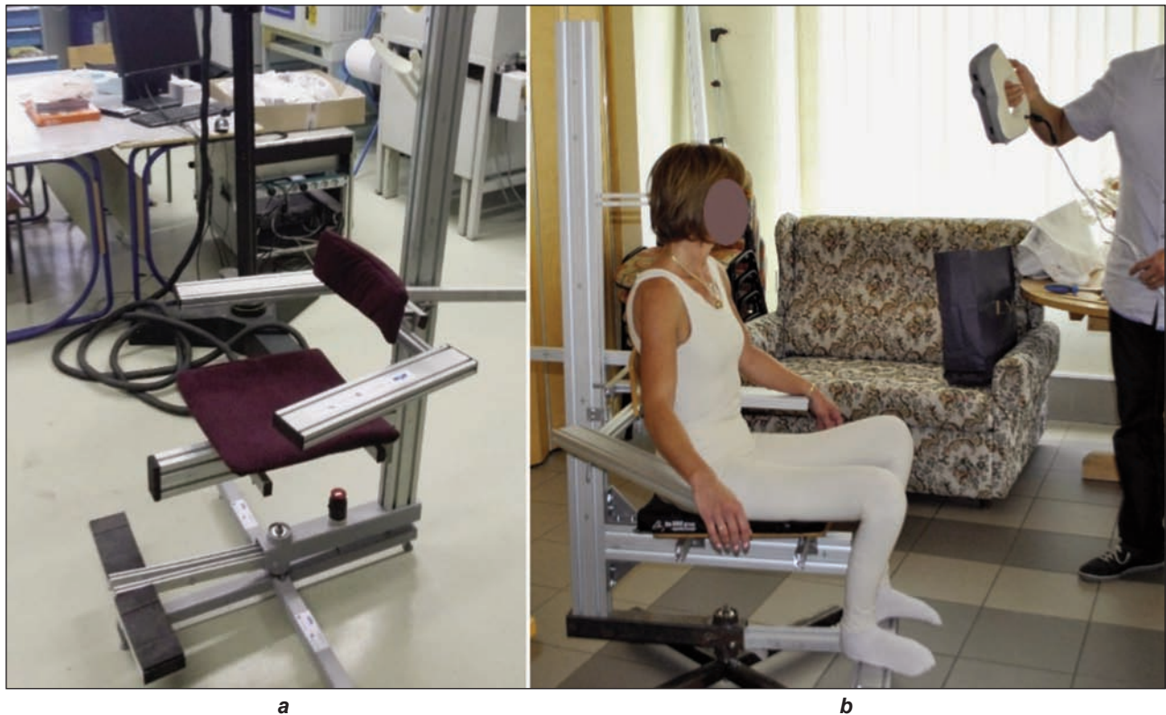
Fig. 1. The chair prototype for scanning of the IMP (a) and application (b)
